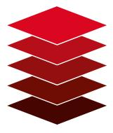
PET Protection Film (50 μm) Protection Film (10 μm) Non Yellowing TPU (175 μm) Adhesive (40 μm) Release Liner (80 μm)
